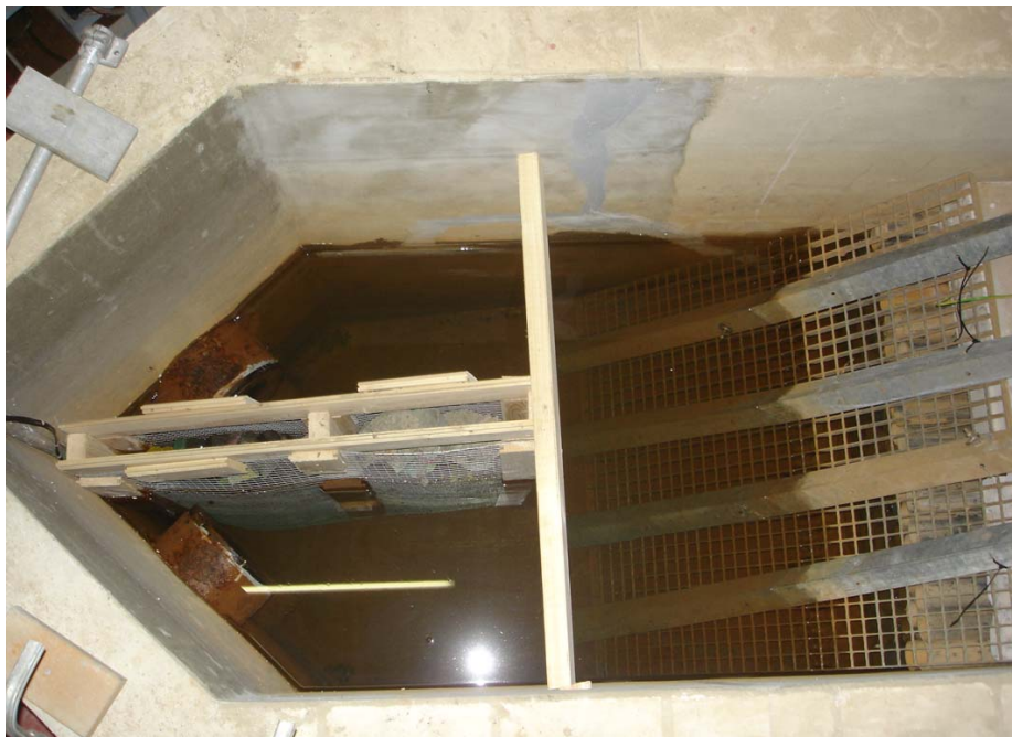
Figure 4.3 Photograph of the flume intake and the calming of the flow by means of a gravel and rock gabion wall and polyethylene tubes
