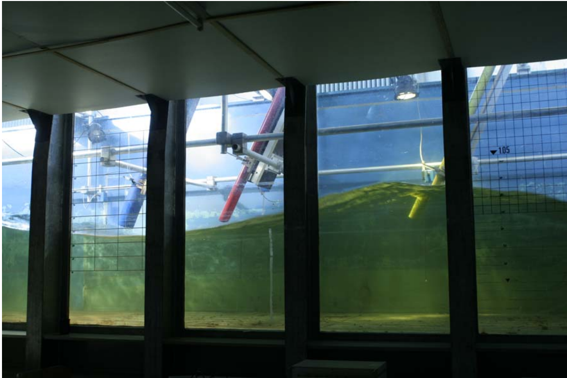
Figure 6: "Wave Tube" Installation in a Laboratory Wave Channel with Large Tube "blue" contra E 1 (38,89 Hz), Medium Tube "red" B 1 (58,26 Hz), Small Tube "yellow" E 1 (77,78 Hz)
