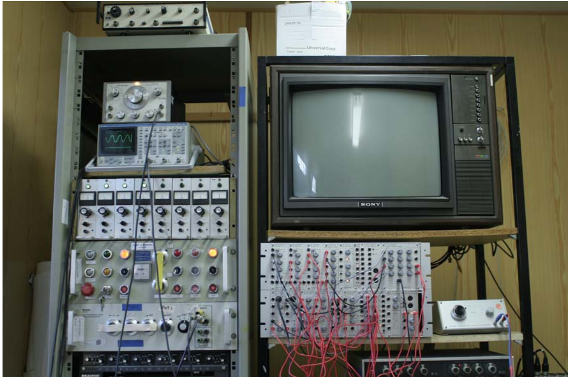
Figure 9: Synthesizer Setup: Analogue Synthesizer Connected to Wave Machine, “Wave Tube” Microphones and Wave Gauges
